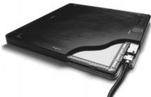
Fig. 2. Flat-panel active-matrix direct-conversion X-ray imager using a-Se as the X-ray to charge transducer with an active area of 14 \times 17 in. (Courtesy of the Direct Radiography Corporation.)
